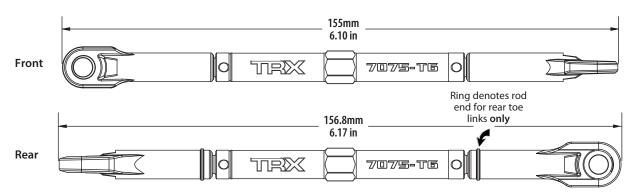
All of the toe links were originally installed on the truck so that the left hand thread indicators point in the same direction. This makes it easier to remember which way to turn the wrench to increase or decrease toe link length (the direction is the same at all four corners). Note that a groove indicates the side of the Tube with the left-hand threads.
